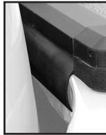
Place dust seal between cab and truck bed.
